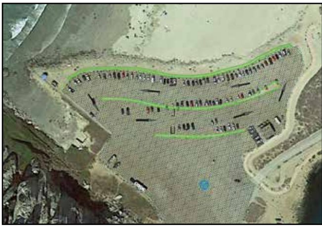
The rendering shows a preliminary layout for linear, bioretention, stormwater catch basins that are being proposed for the Morro Rock parking lot. Renderings courtesy City of Morro Bay
