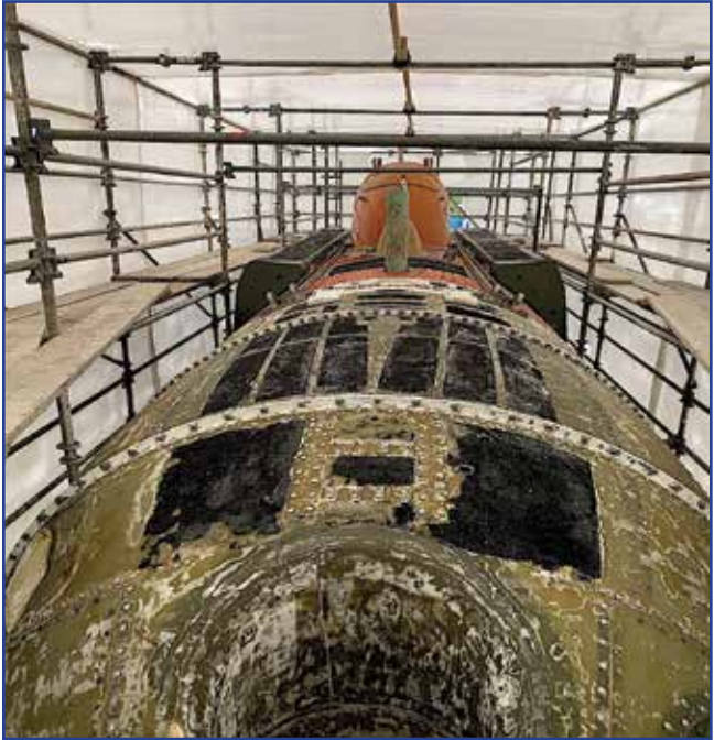
A peek at the top of the DSRV Avalon sitting inside a plastic cocoon so it can be kept dry while being painted.
