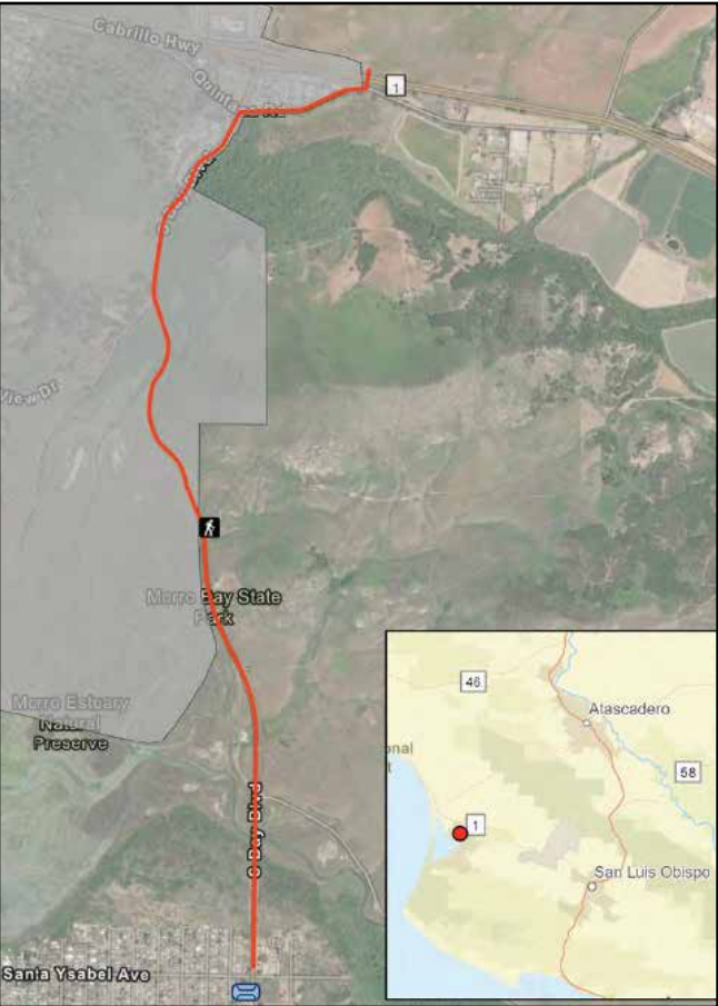
Map shows the route of a proposed water pipeline that would bring state water to Los Osos. The pipeline would follow existing roads [Quintana and South Bay Boulevard] and is depicted in red. The shaded area is the Morro Bay City Limits. The remaining area is under County jurisdiction. Map courtesy LOCSD
