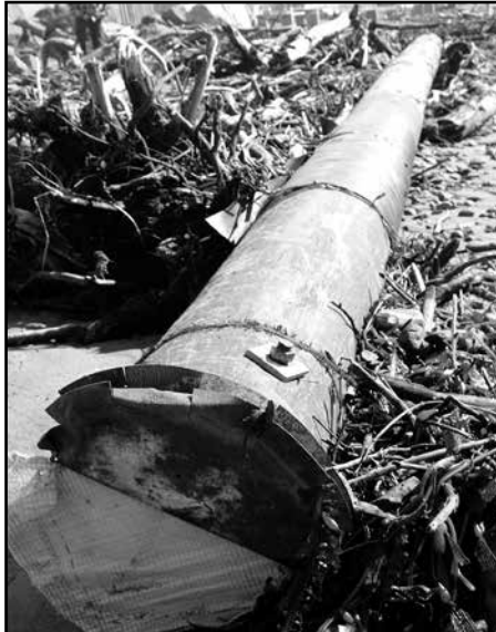
A look at the still wrapped and treated wooden pile that seemed to be entirely intact, lying amongst a mountain of driftwood below the Vet's Hall parking lot.
