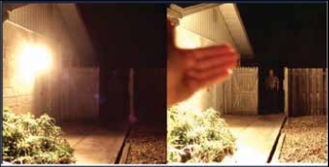
Excessive light does not enhance security. With the light shielded, the figure at the gate becomes visible.
