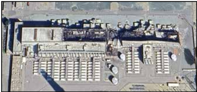
Google Earth image shows the burned-out portion of the Moss Landing BESS that caught fire last January. In the foreground are rows of battery assemblies of Vistra's second battery plant that was untouched by the blaze.
