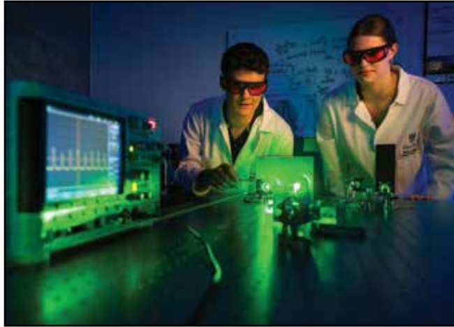
Cal Poly physics students James Mauck and Hannah Bauer align a green light pump laser used as part of a project to build Cal Poly's first laser. A green pump laser excites the crystal, enabling it to emit tunable red and near-infrared light. Photo by Cal Poly Jay Johnston
